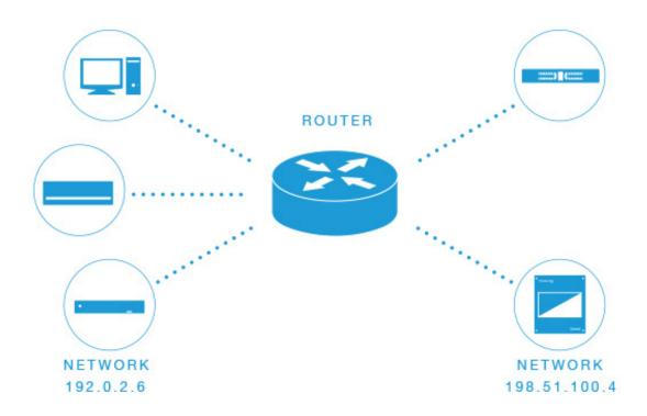
Figure 1. Sample Networking Scenario. For example, if the mDNS gateway functionality is enabled on the router in this figure, then service information can be sent from one subnet to another and vice-versa. For example, the NDI discovery information being advertised in the network with IP address 192.0.2.6 (left) is redistributed to the network with IP address 198.51.100.4 (right) and learned by the mDNS-enabled hosts and devices in that network.
